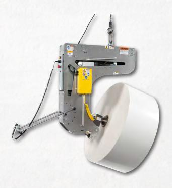
Options for below the hook roll handling units range from light duty (0-500 lbs.), heavy duty (500-5000 lbs.) and super duty (5000 lbs.+). Each has its own advantages for use in a variety of environments.
