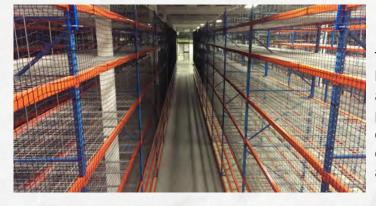
These netting systems sit flush to the racking system, helping to ensure that no product will fall. Ideal for applications where there is no pallet overhang or product is loaded by hand. This system uses the same components as our standard netting, except for the use of flushmount brackets to ensure the netting panel is as close to the rack as possible.
