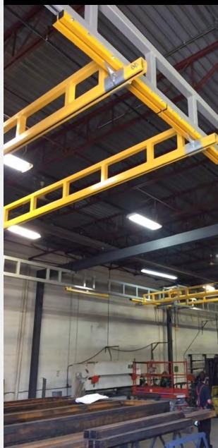
Designed to eliminate manual lifting and enable workers to move loads from workstation to workstation. These systems are ideal for moving loads ranging anywhere from 250 lbs. to 6 tons along a bridge.
