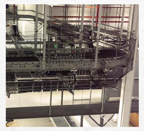
Implementing proper conveyor netting systems will result in an immediate increase in safety throughout your facility. Our netting systems can be customized to every conveyor set-up using various net types that won't rust, peel, rot or dent like metal containment systems. Fine mesh debris liners can also be added for increased protection to workers below.
