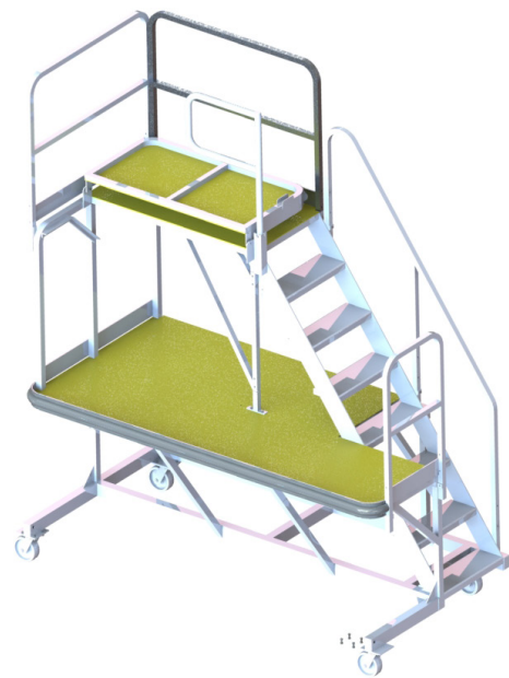
UPPER ACCESS PLATFORM IN FOLDED POSITION
