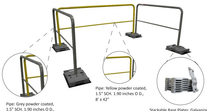
Stackable Base Plates: Galvanized cast steel weights (40 lbs) with three optional holes for vertical post-placement. Includes handles to avoid pinch points. Masticated rubber pad included.
