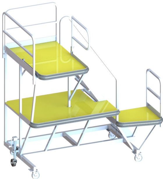
UPPER ACCESS PLATFORM IN EXTENDED POSITION
